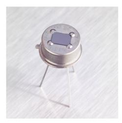
The DigiPyro® PYD 1978, with its 3 x 4 mm<sup>2</sup> window size, provides you with a low-cost digital solution to motion detection.
